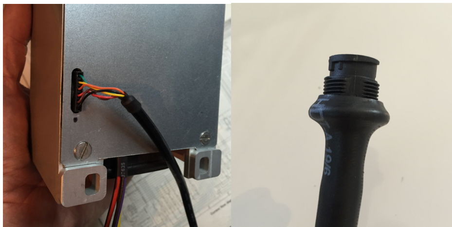
Road unit (left), Race unit waterproof connector(right)
